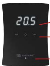
**7-segment display.** Visible when device is activated.
